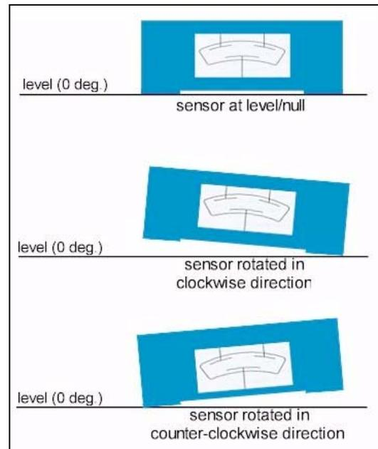
6. Turn 'Sensor Null Adjustment' potentiometer until output on Digital Voltmeter reads 0.000Vdc (see below for potentiometer locations).
