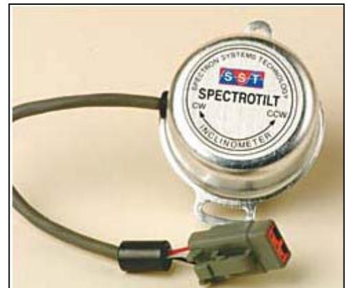
Figure 4. The Spectrotilt RS-232 uses onboard linearity and temperature compensation to eliminate intrinsic measurement errors. The EMI/ESD protection, hermetically sealed sensor, aluminum housing, and fully potted electronics give it immunity to harsh environments.
