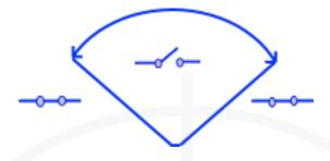
**NC normally opened:** The contact is open before it reaches the trip point. Once the trip point has been reached the contact closes allowing the relay to send a message
