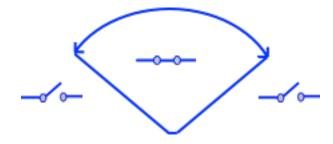
**NC normally closed:** The contact is closed before it reaches the trip point. Once the trip point has been reached the contact opens allowing the relay to send a message
